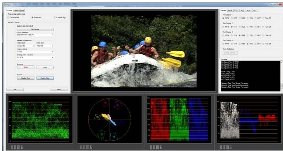
**Figure 1.0 Typical Video Scope layout**
