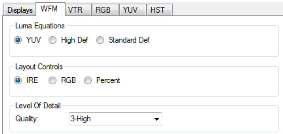
**Figure 5.0 Waveform Monitor Scope operational configuration dialog**
